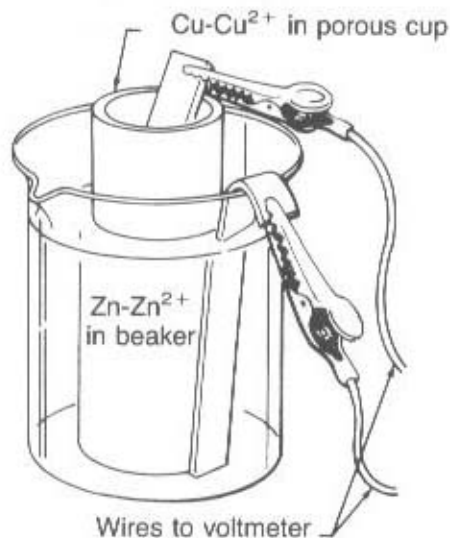
FIGURE 45-2. Copper and zinc half-cells combined.
